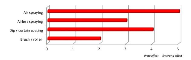
**UNIQ**® **FOAM 280 W** is recommended for high gloss emulsion systems based on acrylate/polyurethane and polyurethane in the pigment volume concentration range 0-25. The additive is effective when used in all traditional application such as rolling, brushing, spraying and pouring.
